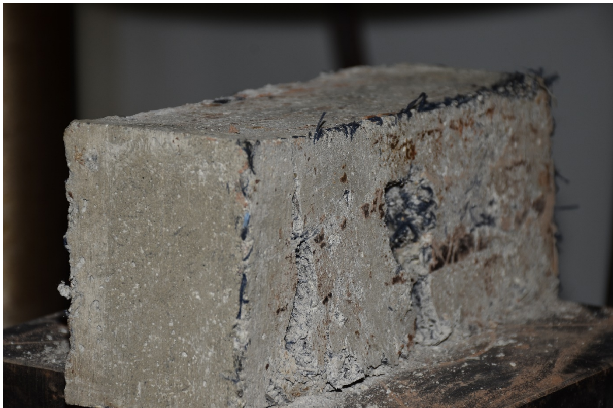
Figure 2. Eco-friendly cement brick integrated with fabric waste produced
