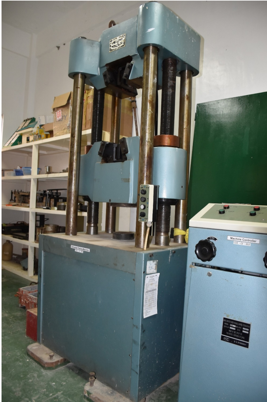
Figure 1. Universal testing machine used in obtaining data on the mechanical properties of the two (2) types of bricks
