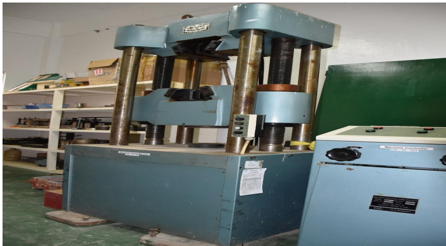
Figure 1: Universal testing machine used in obtaining data on the mechanical properties of the two (2) types of bricks
