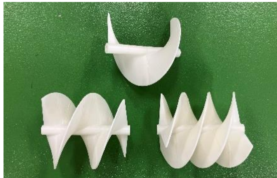
Figure 6: The spiral waterwheel actually built by the authors
