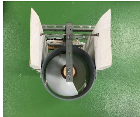
Figure 9: Water diversion prevention mechanism
