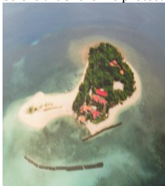
b. Two shorelines protection measures were taken to reduce beach erosion in 2006.
