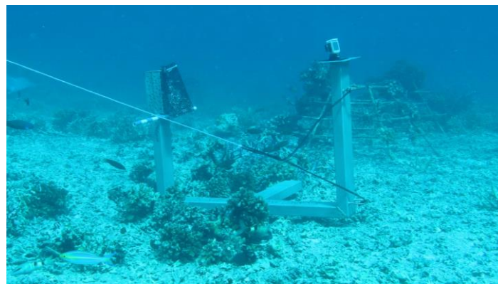
Figure 4. BRUVS steel structure equipped with GoPro Hero 8 camera and a bait's housing at 1 m in front of the camera.
