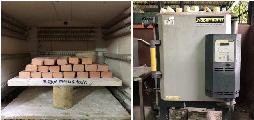
Figure 3 Sample fired in electric kiln
