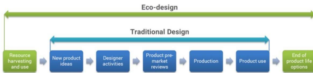
Figure 5: A conceptual model of traditional and eco-design processes for furniture product development.
