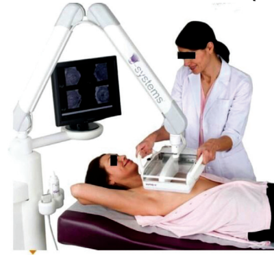
Figure 3 Automated breast ultrasound (ABUS)
