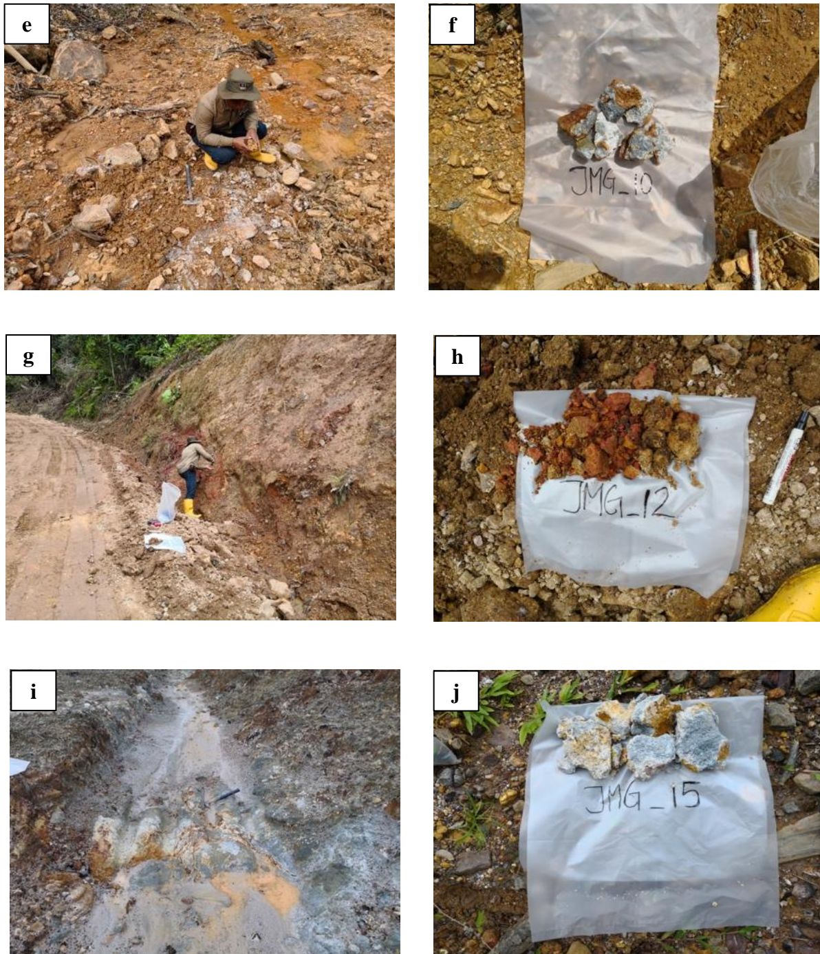
Figure 2. Outcrops and hand specimen samples in the alteration zone of andesite and volcanic breccia in Bukit Mantri area; (a) and (b) argillised andesite, (c) and (d) propylitised andesite, (e) and (f) silicified andesite, (g) and (h) volcanic breccia, and (i) and (j) argillised and sulphidised andesite.
