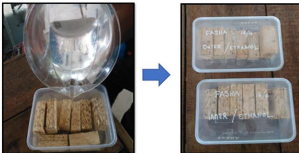
Figure 2. The soaking treatment process of cube-sized oil palm trunk (OPT) with ethanol. The samples were kept in a closed container at room temperature for 24 hours before drying.
