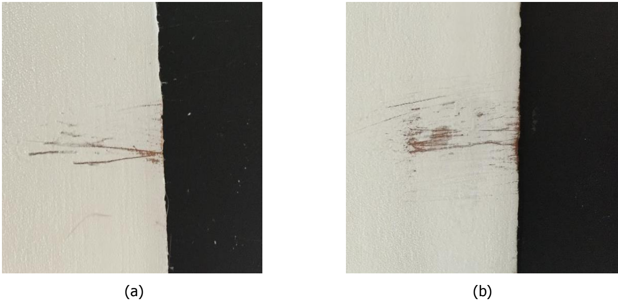
Figure 4: Abrasion resistance on the (a) AMCA lacquer is higher than the (b) CCA lacquer, with 288 and 271 cycles, respectively.
