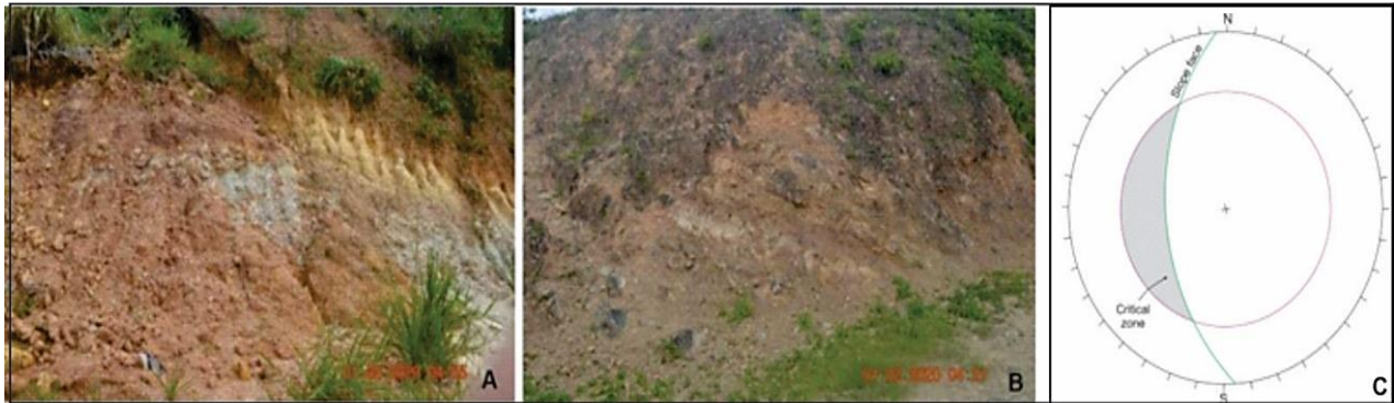
Figure 7 The weathered (class IV) rock unit. A- Crocker formation; B- Trusmadi formation; C- planar failure.
