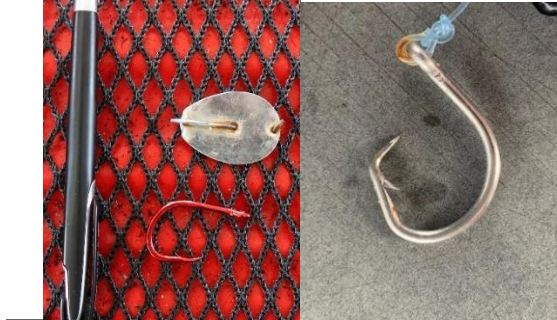
Hook – attaches to the tuna's mouth when the bait is taken. Coin-shaped bait – used with J-shaped hooks; the shiny, reflective surface attracts the attention of tuna.
