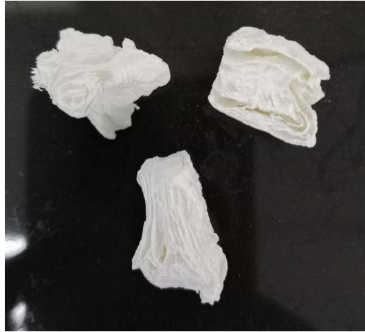
Figure 1. Cross-sectional image of the chitosan/TiO 2 composite membrane showing the porous sponge-like architecture generated after freeze-drying.
