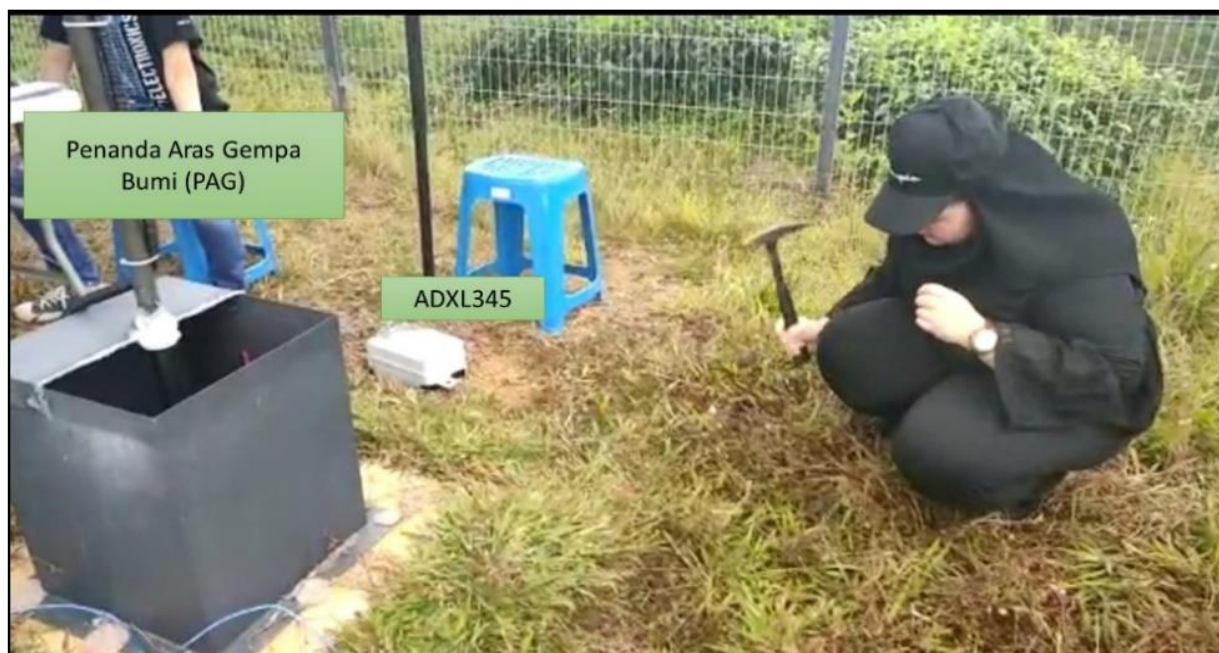
Figure 2: Placement of PAG and ADXL345 is in distance 1.0m and force is given from 3.0m away of both devices.
