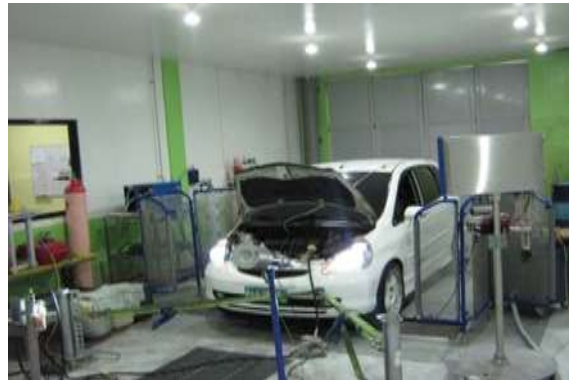
Figure 3: Vehicle-chassis dynamometer set-up
