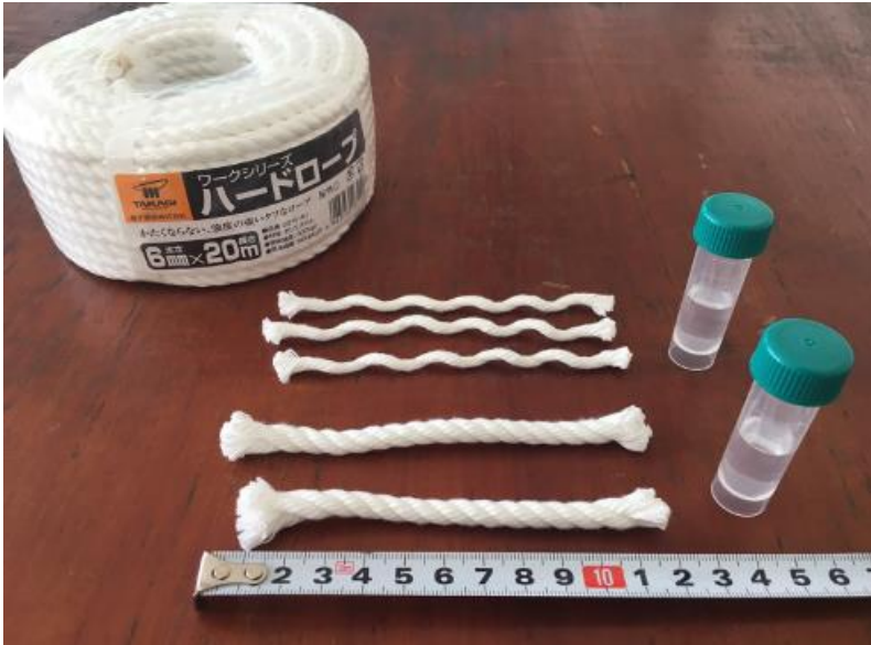
Figure 1. Rope swabs cut into 10cm length and 3ml of lysis buffer in 5ml tube
